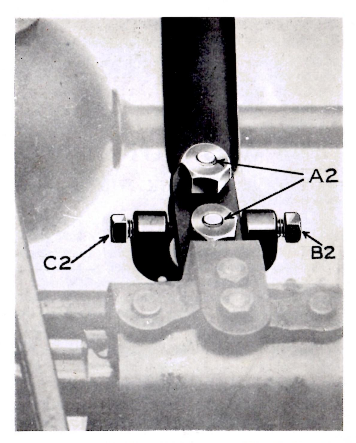
If, however, YOU OVER-ADJUST THE CLUTCH SO THAT A "FREE ENGINE" IS NOT OBTAINED when the clutch lever is in the "out" position, reverse the operation, i.e., slack back screw (B2) and tighten up screw (C2), finally ocking up nuts (A2).
