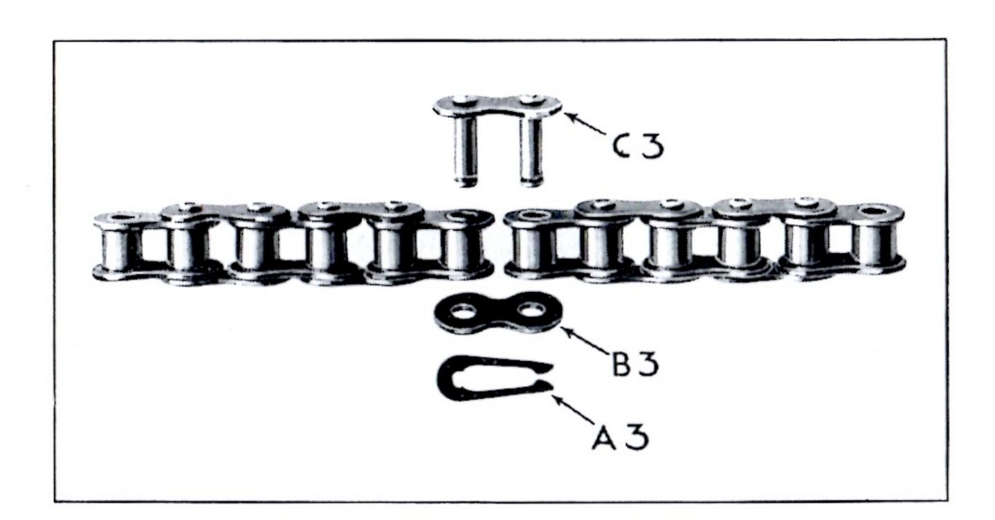
NOTE.—When replacing the chains be sure and fit the spring link so that it is pushed into place the reverse way to the direction of motion of the chain when working.
