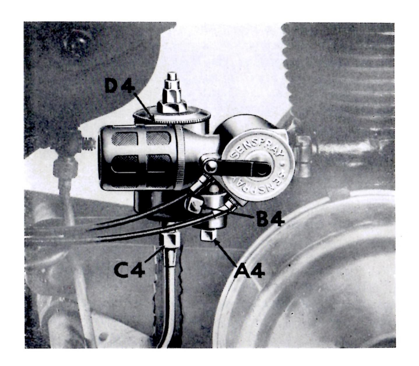
If there is dirt inside the jet it will be advisable to examine and clean out the inside of the float chamber at the same time. Unscrew petrol pipe union nut (C4) and remove float chamber cap (D4). Gently pinch together the ends of the valve spring clip (A5) as illustrated (below), when it may easily be drawn off the valve stem. The valve (B5) may then be slipped out downwards and the
