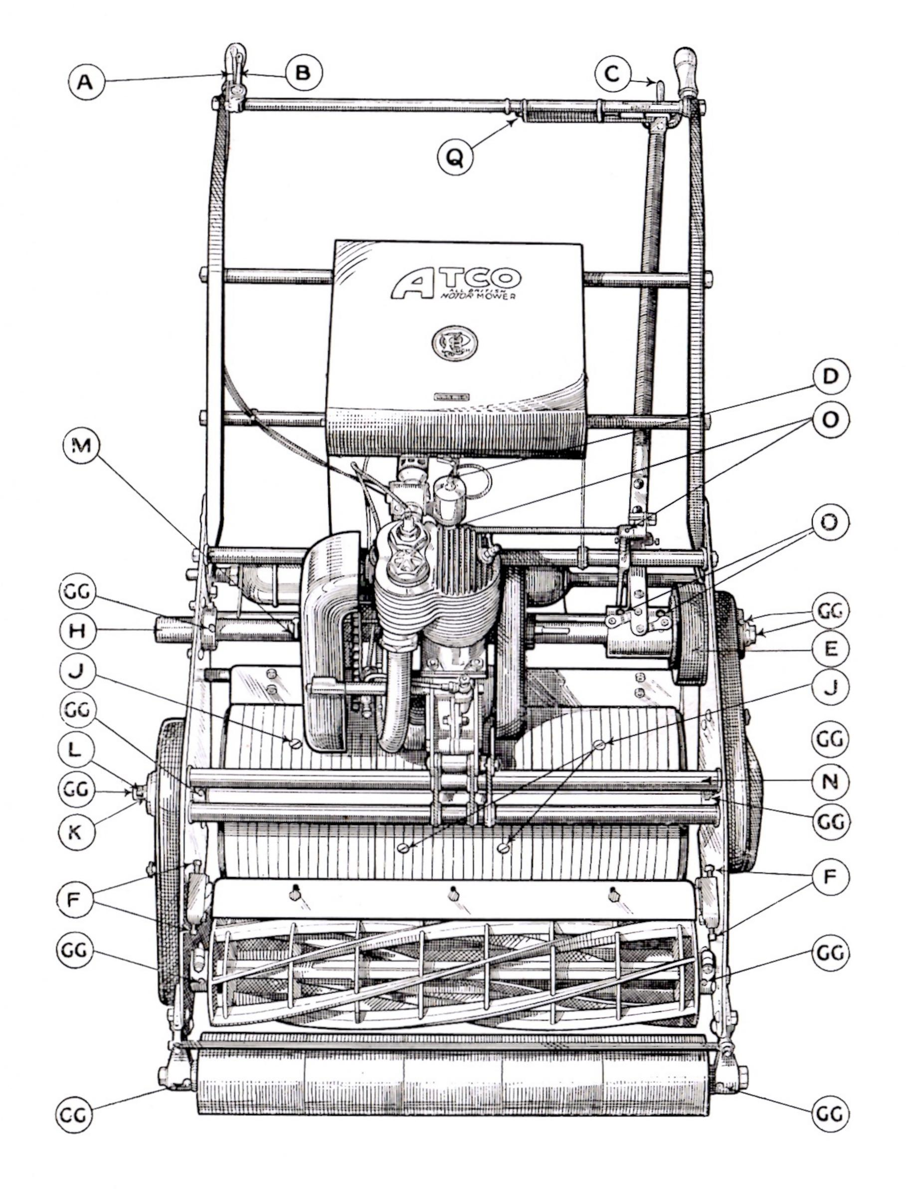
TO TIGHTEN THE MAGNETO CHAIN, the four square-headed set screws underneath the base of the magneto must be slackened off. The magneto can then be moved bodily along in its guide until the chain is just nicely free, when the four screws must be tightened up again, CAREFULLY, WITHOUT USING UNDUE STRENGTH.
