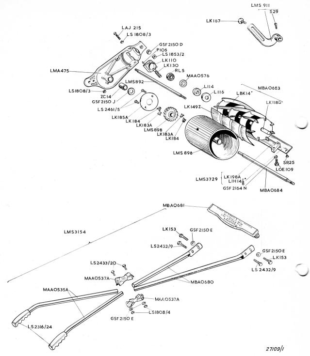
The above are "exploded" views of the "Ascot" mower showing clearly all the component parts and the part numbers, and the descriptions are given on pages 6 and 7.
