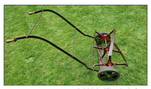
At first glance this piece of machinery may appear to be some sort of reaper, however it was designed for the more delicate operation of cutting 'Bents' on fine turf, golf greens etc. The 'Bents' referred to being the long, tough, grassy stems which escape the ordinary lawn mower.
