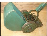
en rear roller, which is a three piece affair on a central shaft like a more expensive roller mower version. Original wooden rollers also have a concave shaping to the corners. something not seen elsewhere. The cutting cylinder is unusual too, the central spider (earlier 12 inch models have two spiders) holding the blades is floating rather than attached to the shaft.
