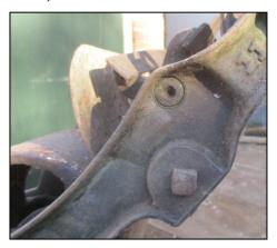
The cheapest way of arranging a bearing must surely be that found on a Follows & Bate Tennis. *(see right)* This type has no fine adjustment screws at all with the cast iron bearing block just sliding up and down in a slot on the frame, and the securing bolt being tightened when you've managed to get it to about the right place. As an aside, This machine must win awards for being one of the worst mowers ever sold, not only is the bearing design awful, but the gear
