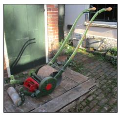
cover on the cylinder pinion end offers no scope for adjustment so it can't be tightened up without the pinion scraping on it. Even if you overcame these two problems, this specific example had a party piece to prevent it ever having seen much use. Out of the five blades in the cylinder three have been put in back wards so that the soft wrought iron edge is leading and the hardened cutting edge is uselessly trailing.
