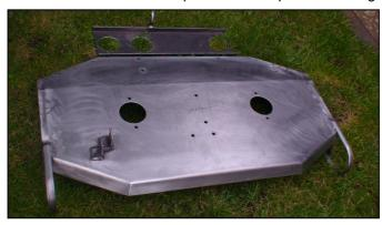
These were pitted and buckled comas under pressed the wood pile, so unbalanced and bevond use, so I made new bosses using a large hole saw and using a Jones & Sweeney Fly press, pressed the blade rotor plates.
