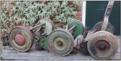
Three different Magics; Left, the later (post War) S2 version, a basic Magic in the centre and on the right a Magic sold by BHAT (see text right). The latter machine has a very basic and crude adjustment system which must have made it virtually impossible to set it to cut properly.
