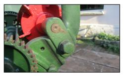
no slack in the slot as this can have the same effect as slack in the bearing itself.
