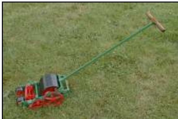
This Ransomes Reversible, belonging to Stan Hardwick, won the Andrew Grout Plate at the Annual Rally in 2003. The mower was called the Reversible because the whole chassis could be inverted and the bottom-block and handle repositioned so that the leading edges of the blades, blunted by use, became the trailing edges. The idea was that they would be re-sharpened automatically while the sharp, previously trailing edges, were doing their turn as leaders. The machine dates from the late 1870s to early '80s. A similar, simpler idea was employed on the Silens Messor where the cutting cylinder could be reversed to achieve the same self-sharpening effect.
