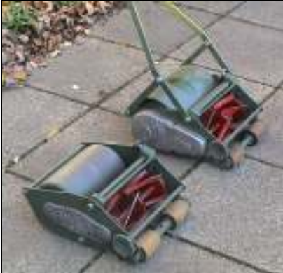
These JP Minors, slightly different designs, are part of Henry Ellis's collection. The one on the left was introduced in 1930 and was replaced by the one on the right in 1936. Henry, one of our JP aficionados, has recently confirmed that post WW2 JPs were painted with colour close to BS381 C223 Medium Bronze Green and from 1961 with colour close to BS381 C222 Light Bronze Green.
