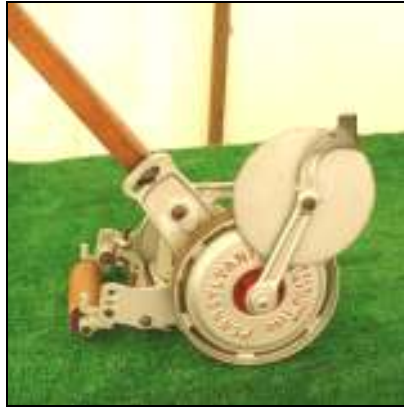
Alan and Dick Hardwick showed this unusual Pennsylvania edger at Banbury Steam Rally. The large disc is for trimming the edge of the lawn.
