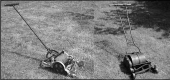
In those machines which collect, an iron box or tray is fixed in front of the knife frame, to receive the cut grass when flung up by the knives. There are also, generally, rollers in front of the knife-frame, which serve to guide the machine, and also to press down the grass into that position in which it can be most easily severed by the knives.
